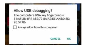
As soon as the it is allowed, you will be able to see the interface of the device into your virtual remote or in service management, you can test again adb and see it "online". If the operation failed, a deep reboot (pressing the reboot button of the virtual remote) and opening again the virtual remote will request again for adb connection.
