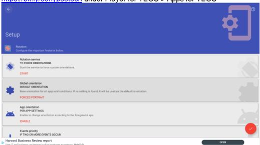
In case rotation is activated please also create an action schedule which will start the Signage application after the daily reboot, this because after a reboot the Signage app and the Rotation app are both automatically starting. In case the Signage app has started earlier it will not use the correct resolution, with the action schedule you can make sure that it does.
