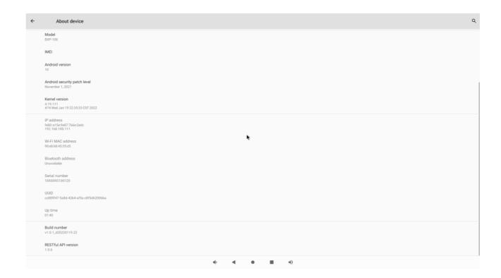
Go back to settings and developer options and enable stay awake and enable ADB and ADB over TCP-IP (port 5555)
